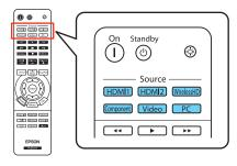
If you press the  $\rightarrow$  source button on the projector, you see a list of available sources. Press the  $\rightarrow$  source button to move through the list and select the desired source.
